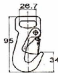
MH04-151A 1" Snap Hook, American Type B/S: 1500Kgs/ 3300Lbs
